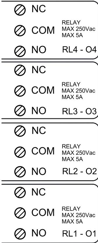
USCITE DIGITALI: n°4 relay in scambio SPDT 5A / 250V<sub>AC</sub>
